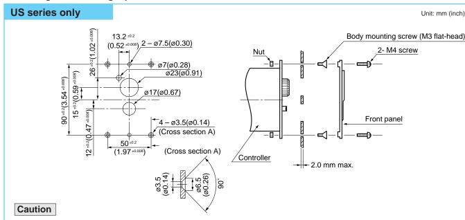
Wall thickness of the equipment where the controller is to be mounted should be 2 mm or less.
